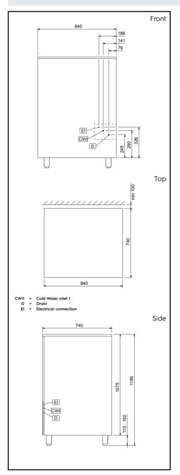
**Electric** Supply voltage: 730531 (RIMC143SA) 220-240 V/1N ph/50 Hz Electrical power: 1.05 kW Capacity: Bin capacity: 65 kg **Key Information:** External dimensions, Height: 1185 mm External dimensions, Width: 840 mm External dimensions, Depth: 740 mm Net weight: 113 kg Output: 130 kg/day Kind of cube: Ice Cube 18 g **Refrigeration Data** R404a
