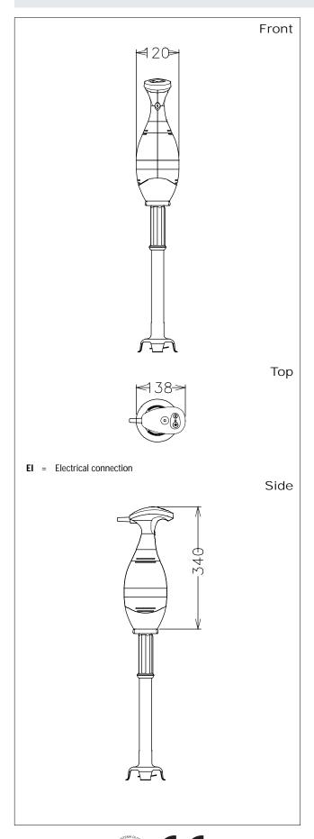
Electric Supply voltage: 603787 (BMX750T65) 220...240 V/1N ph/50/60 Hz **Connected load:** 0.75 kW **Total Watts:** 0.75 kW Capacity: Capacity (up to): 290 liter Key Information: **External dimensions, Height:** 965 mm **External dimensions, Width:** 138 mm **External dimensions, Depth:** 120 mm Shipping weight: 5 kg
