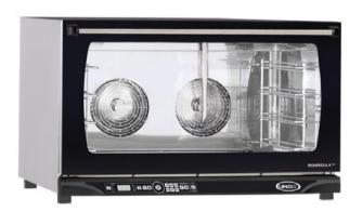
Capacity Pitch Frequency Voltage Electrical power Dimensions Weight XFT195 4 600x400 75 mm 50 / 60 Hz 230 V~ 1N / 400 V~ 3N 6,5 kW 800x770x509 mm 49 kg
